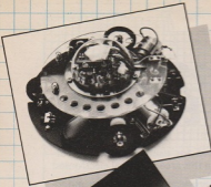
Line Tracer II £17.99 Draw a line and the infra-red sensor picks it up and sends this 3 wheeled, twin motor robot along the course you plot.
